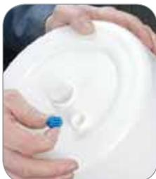
D) Insert rubber plug (5.) into the blue valve cap (4.) if not already assembled like this. Place this piece (rubber part first) into the small round hole in the base of the white pail (3.).
